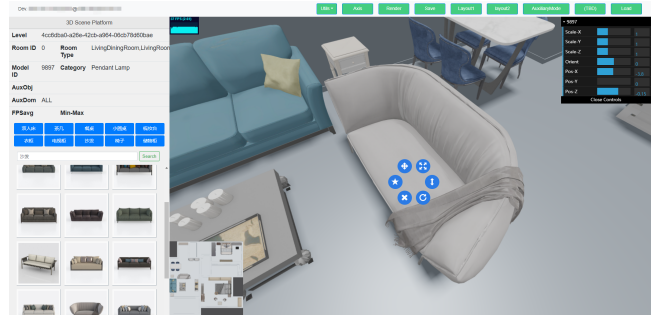
Figure 7: Manipulating objects. Objects can be manipulated by a roulette (Middle) or a panel (Top-Right), including translation, rotation and scale on three axis respectively. The former is more intuitive, where objects are transformed following the cursor. The latter is more numeric, where objects are set according to specific values.
