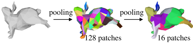
Fig. 3. The hierarchical architecture. The face patches inherit connection relationships from original meshes, which enables them to be continuously processed by the pooling operation to generate new patches from previous face patches.
